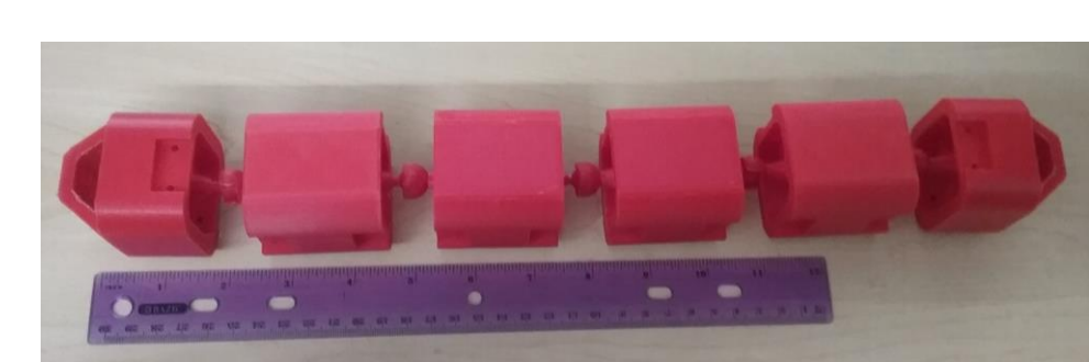
Figure 4: Prototype chassis for the robotic platform. The material used is Polylactic Acid (PLA).
