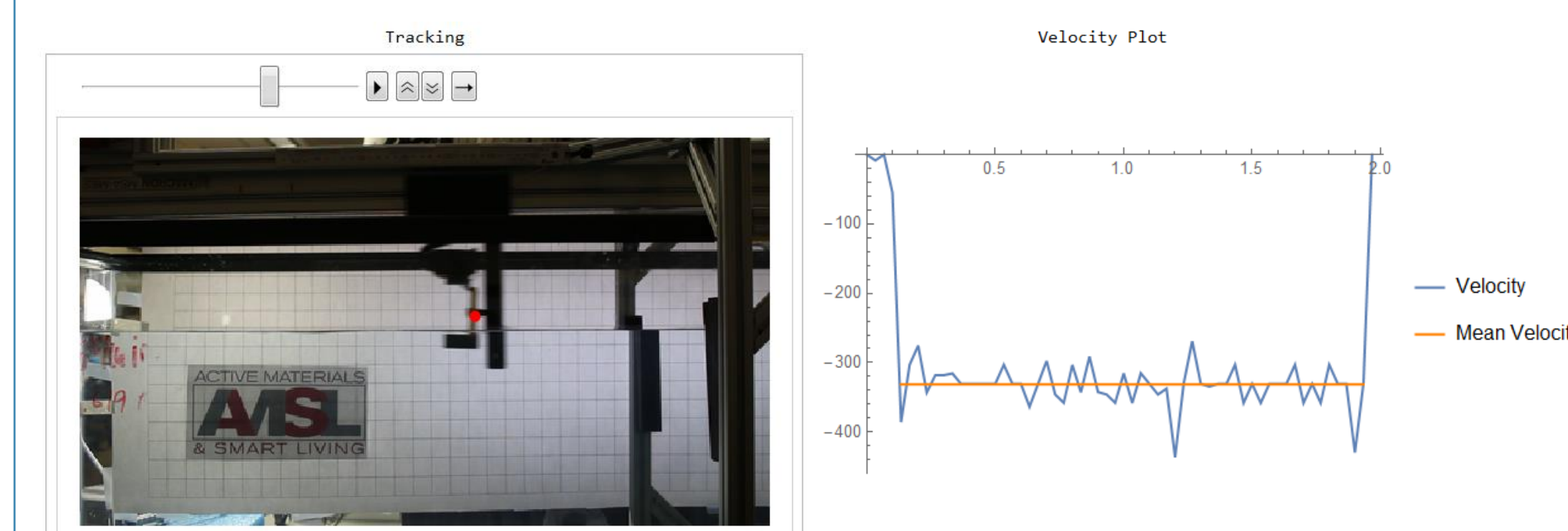
Fig. 3 (Left) Still-frame of velocity tracking footage with centroid of the clamp highlighted by the red dot. (Right) Plotted velocity data along with calculated mean velocity (330 mm/s).
