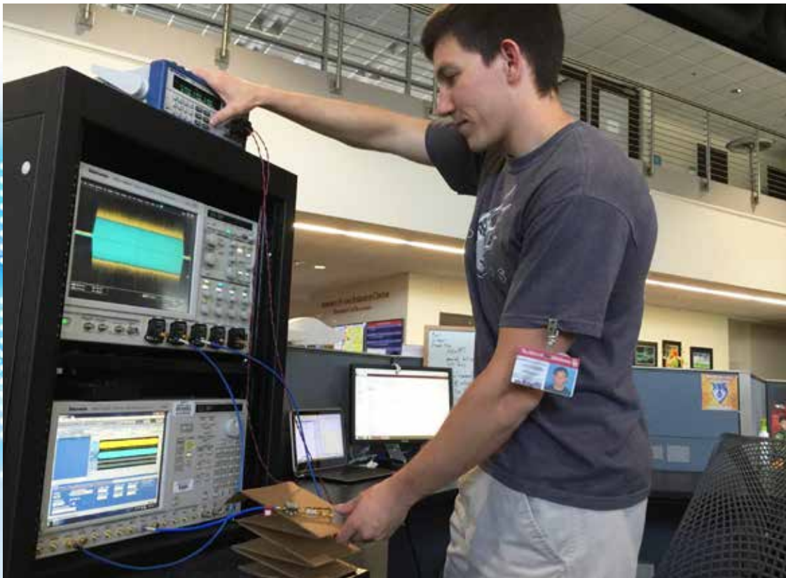
Hands-on, student-led laboratory measurements of radar waveforms at the Radar Innovations Lab at OU confirm our success with the new digital predistortion methods that are needed for the next-generation of phased array radars.
