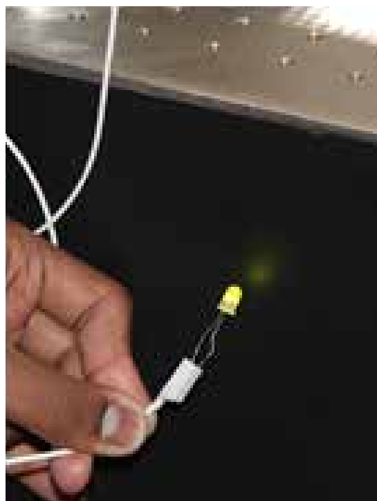
An LED powered by InAs quantum dots solar cells fabricated in the PI-Lab.
