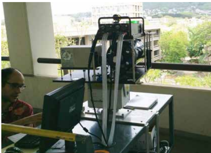
Remote Raman detection of minerals from 430 meters distance with 1 second integration. (Ph.D. Student seen in the image is Tayro Acosta-Maeda and is expected to graduate in Aug. 2016).
