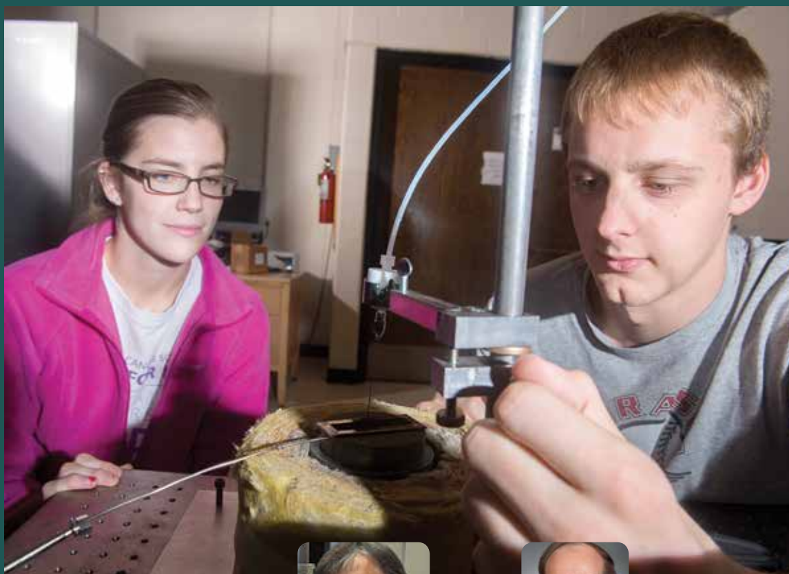
Sarah Wallis (left) and Anton Hassebrook (right) working on an experiment to study the heat transfer characteristics of a metal surface functionalized using femtosecond laser surface processing.
