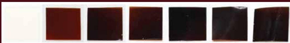
Figure 1: Optimized Nafion®/PI blends ranging from 6 wt% PI (NPI 6) to 30 wt% PI. Nafion® on left.
