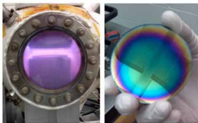
1. The Ar/o-carborane plasma, at left, and a Si wafer with 177nm of boron carbide deposited on it at right.
