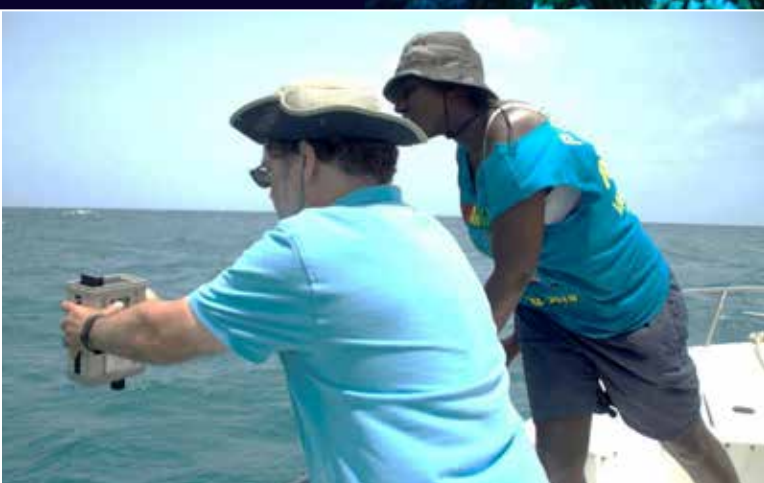
Figure A. Dr. Joseph Ortiz demonstrates to University of the Virgin Islands undergraduate Tia Rabsatt how to use a GER 1500 spectroradiometer to collect data on the optical properties of the water above a coral reef near St. Thomas, US Virgin Islands.
