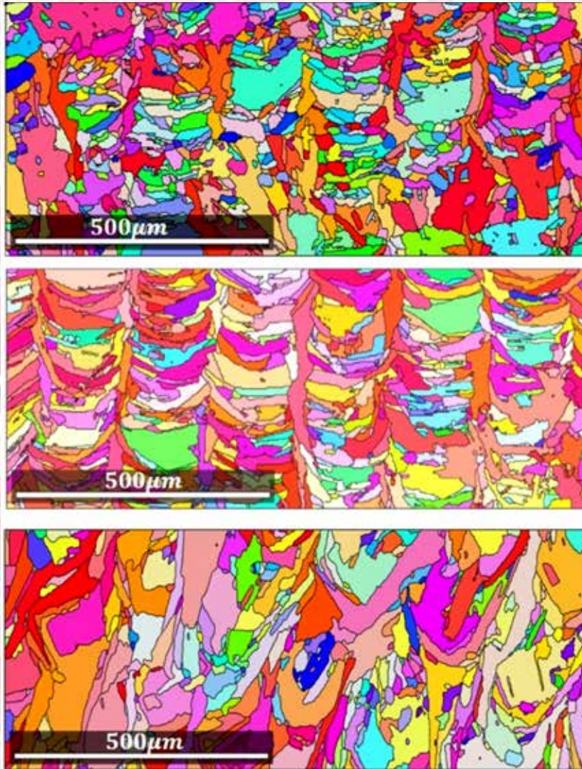
Top: the EBSD results of as-fabricated sample parallel to the build direction of the top, middle, and bottom sections of the sample. Images display the spatial heterogeneity of the as-built SLM parts. Above right: Dr. Lin Li and a student analyze EBSD data of SLM Inconel 718.
