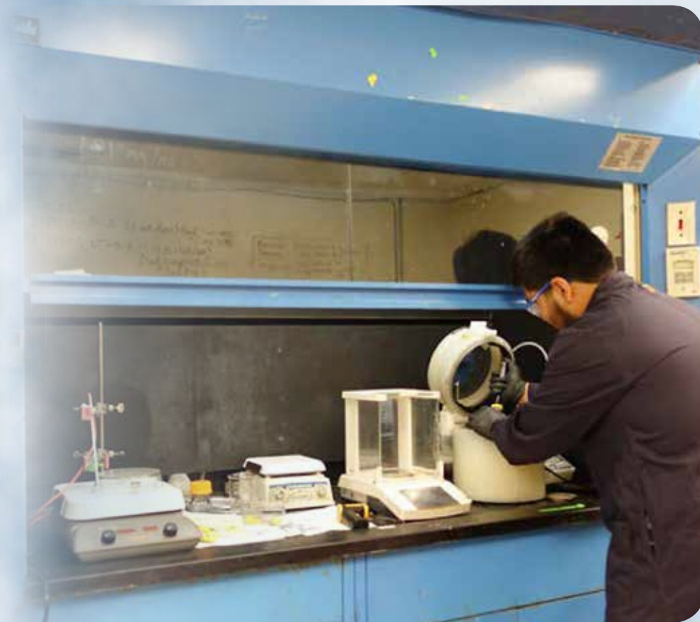
A student is working in LaSMaS at NMT to fabricate MLO composites. He is using a spin-coater for fabricating corrugated P3HT-based self-sensing thin films on PDMS.
