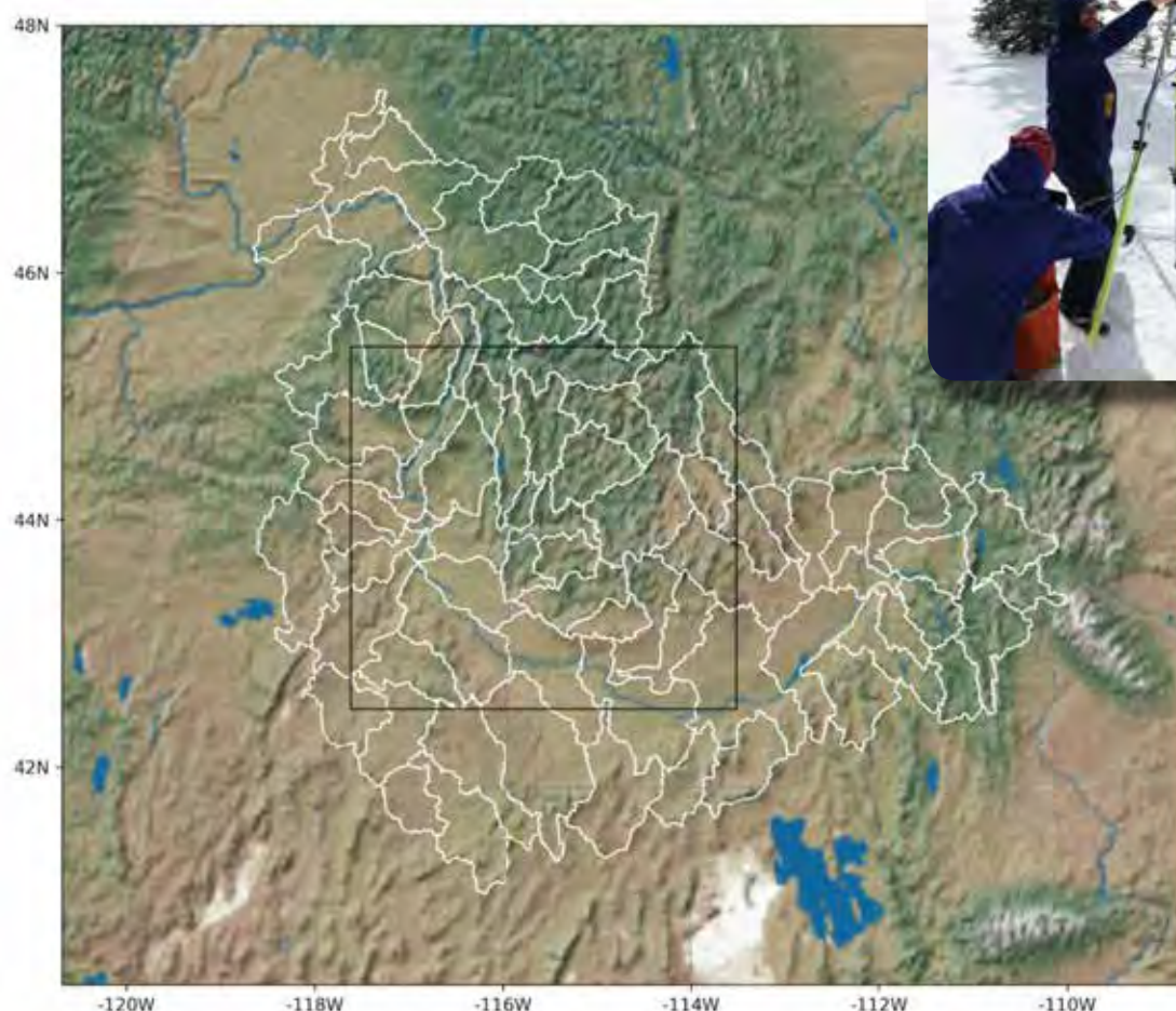
The spatial domains of the land-atmosphere simulator. The outer domain encompasses the entirety of the Snake River Basin (subbasins shown outlined in white) and is associated with a spatial resolution of 3 km. The inner domain, outlined in black, is associated with a spatial resolution of 1 km.
