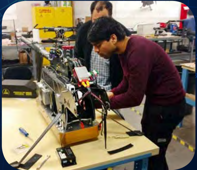
Project collaborators installing the radar antenna on a UAS
