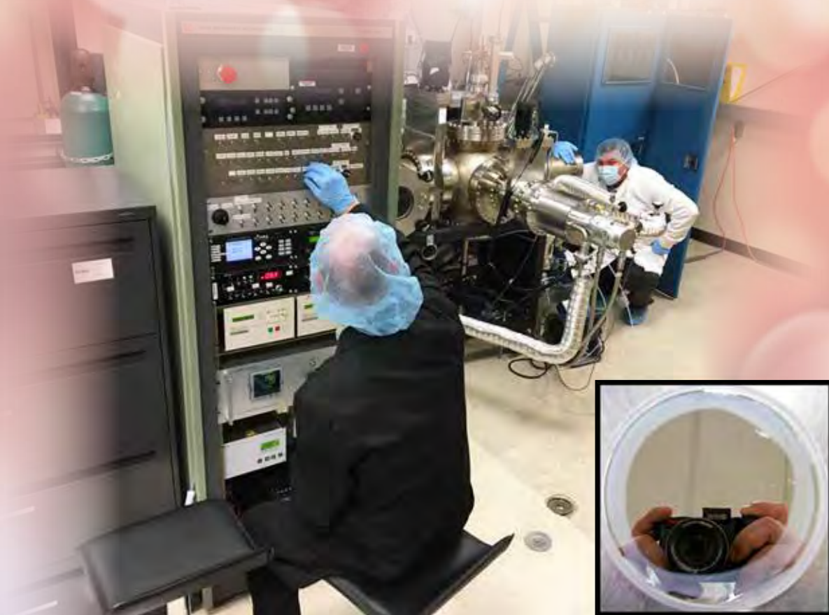
Graduate student researchers working in lab for GeSn film deposition (Inset: a four inch GeSn wafer produced in the lab)
