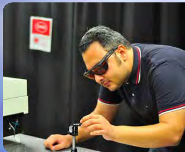
University of Wyoming Ph.D. candidate prepares optics for formaldehyde PLIF visualization of heptane cool flames
