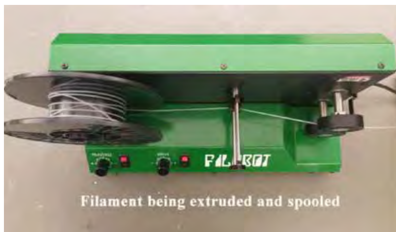
Filament extrusion set up (top and side views)
