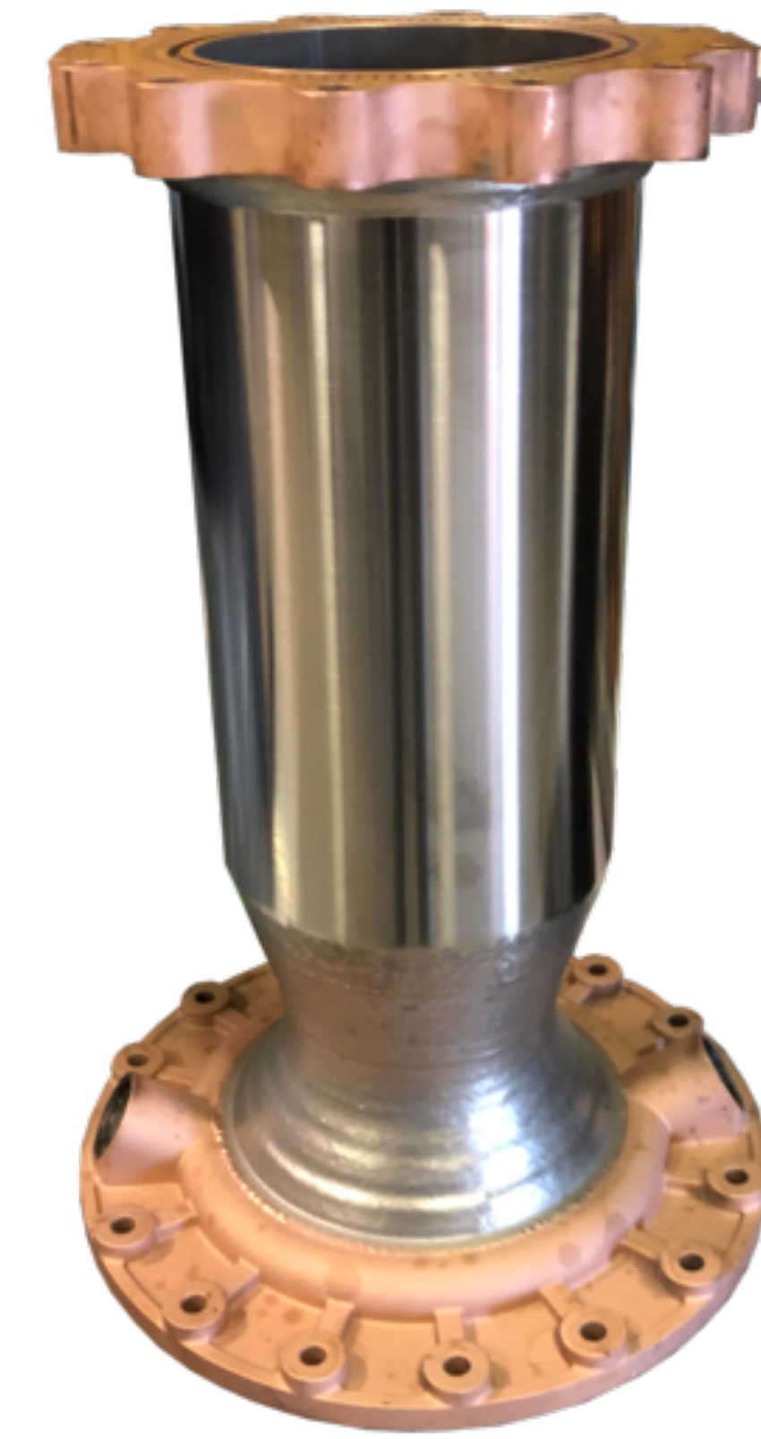
Figure (above): 3D printed thrust chamber. Credit NASA
