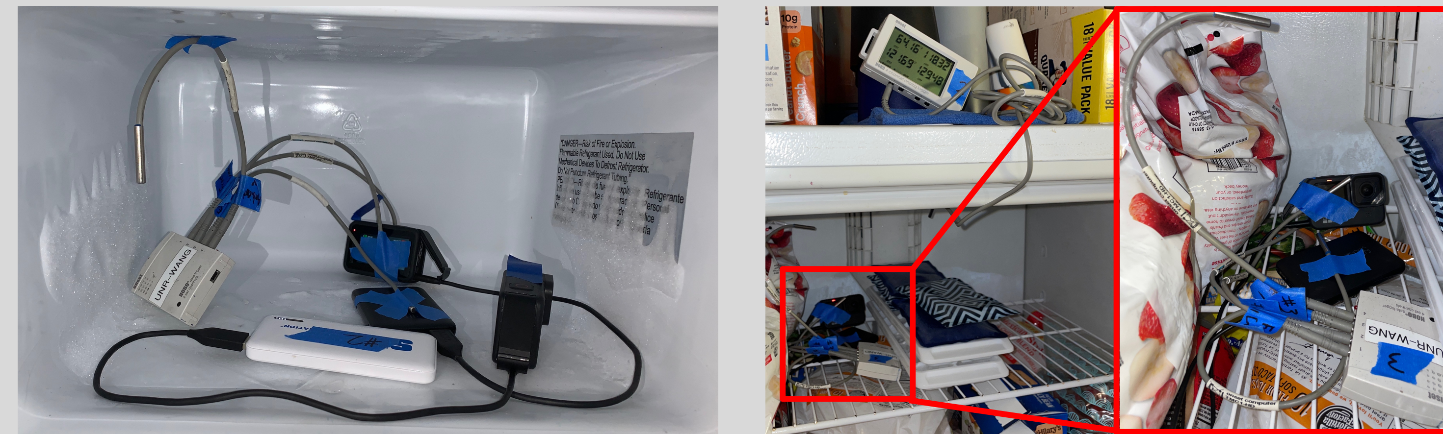
Preliminary tests done in residential freezers
