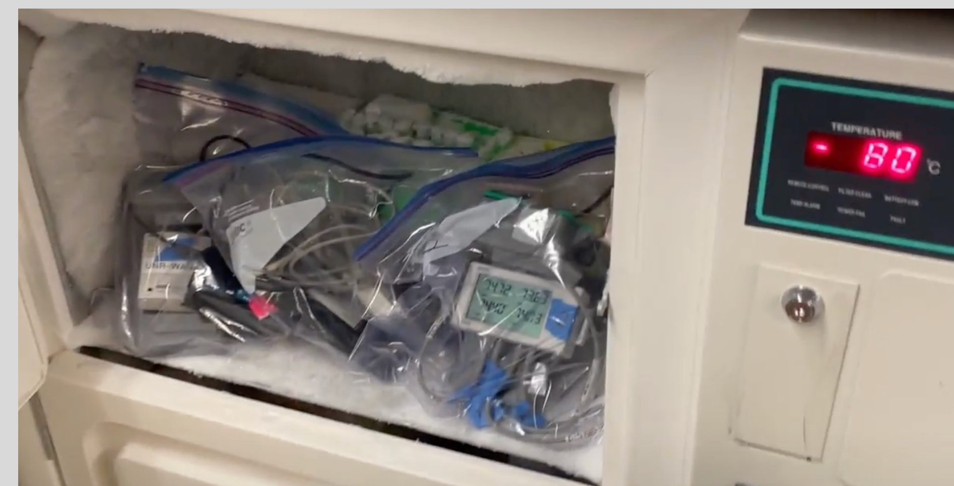
Multiple camera configurations in an industrial-grade freezer
