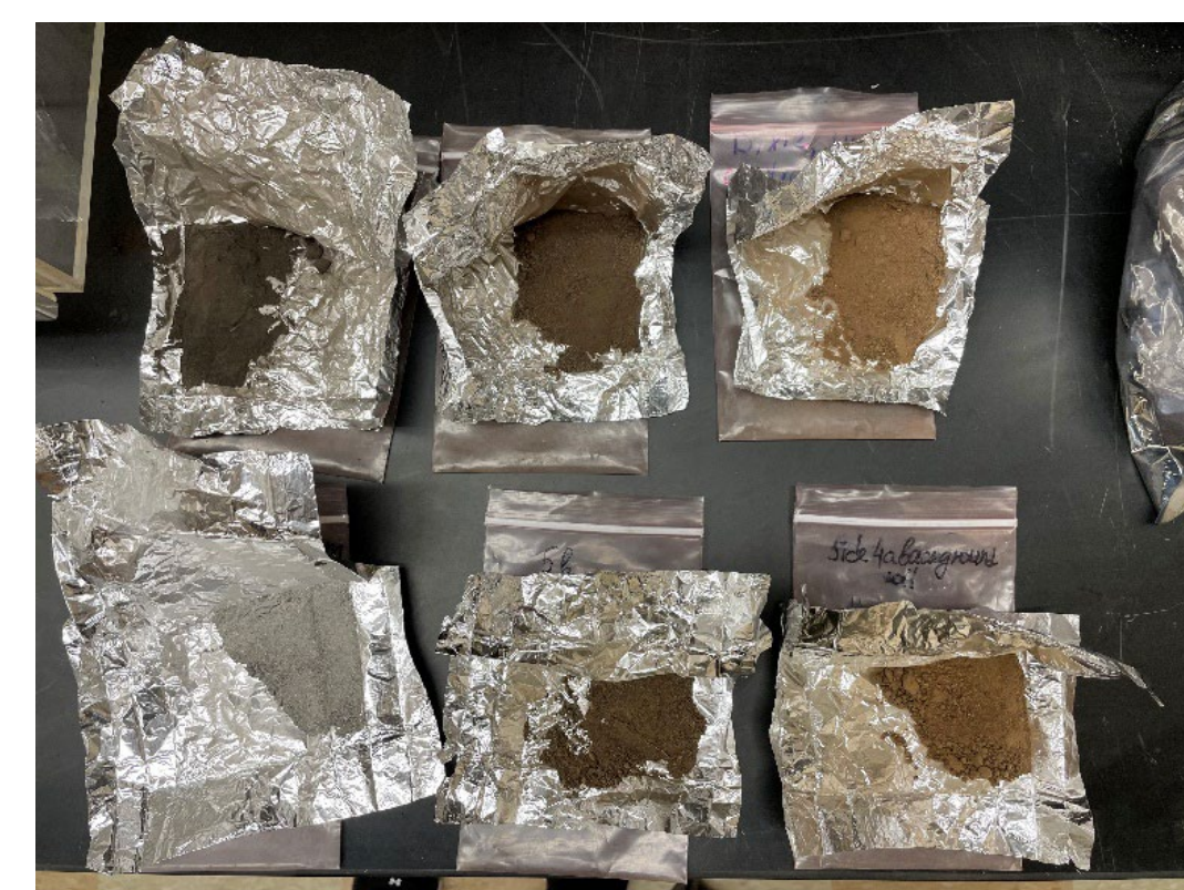
Figure 4. Soil samples (top row collected in 2022, from left to right: ash, burned and unburned, bottom row collected in 2021, from left to right: ash, burned and unburned)
