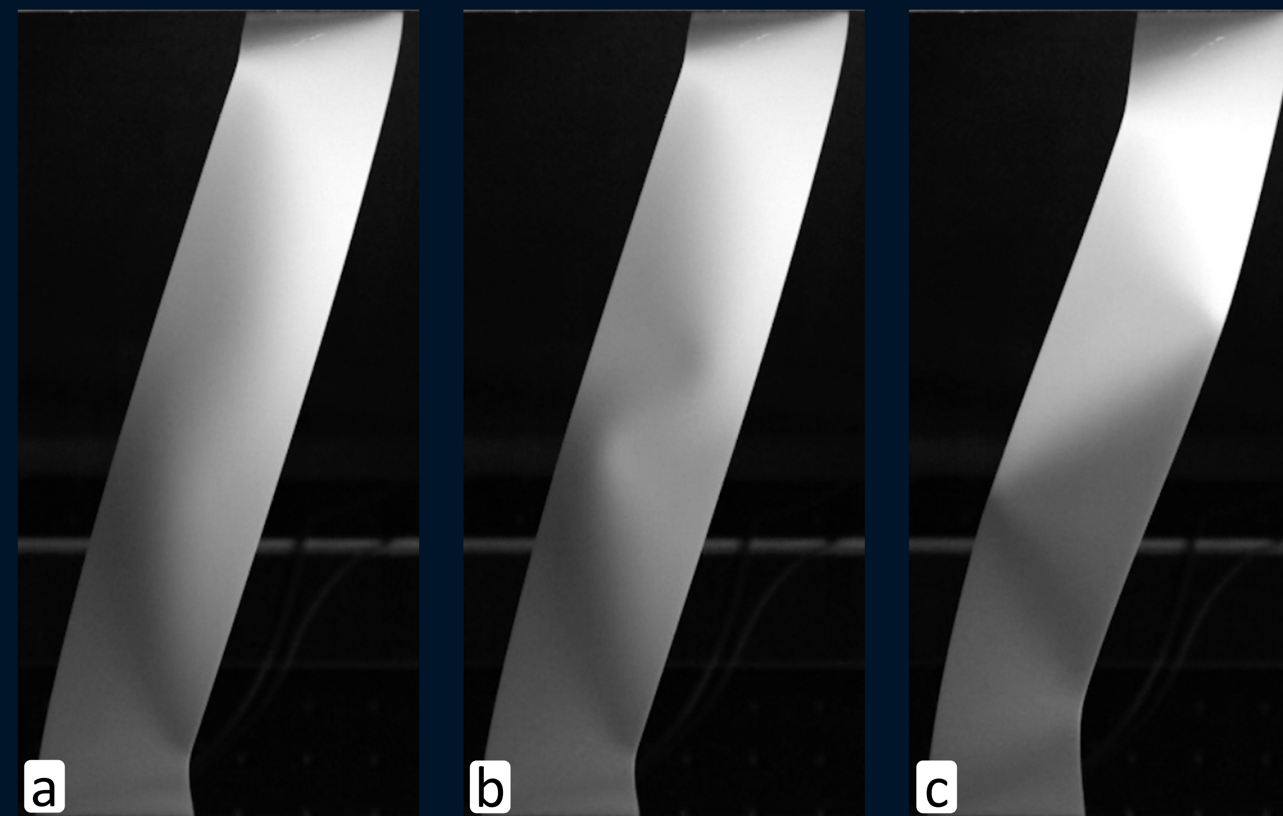
A sheet characterized by \alpha = 0.175 in the pre-buckling state (a), under transient crumpling (b), and post-snap-through state (c)
