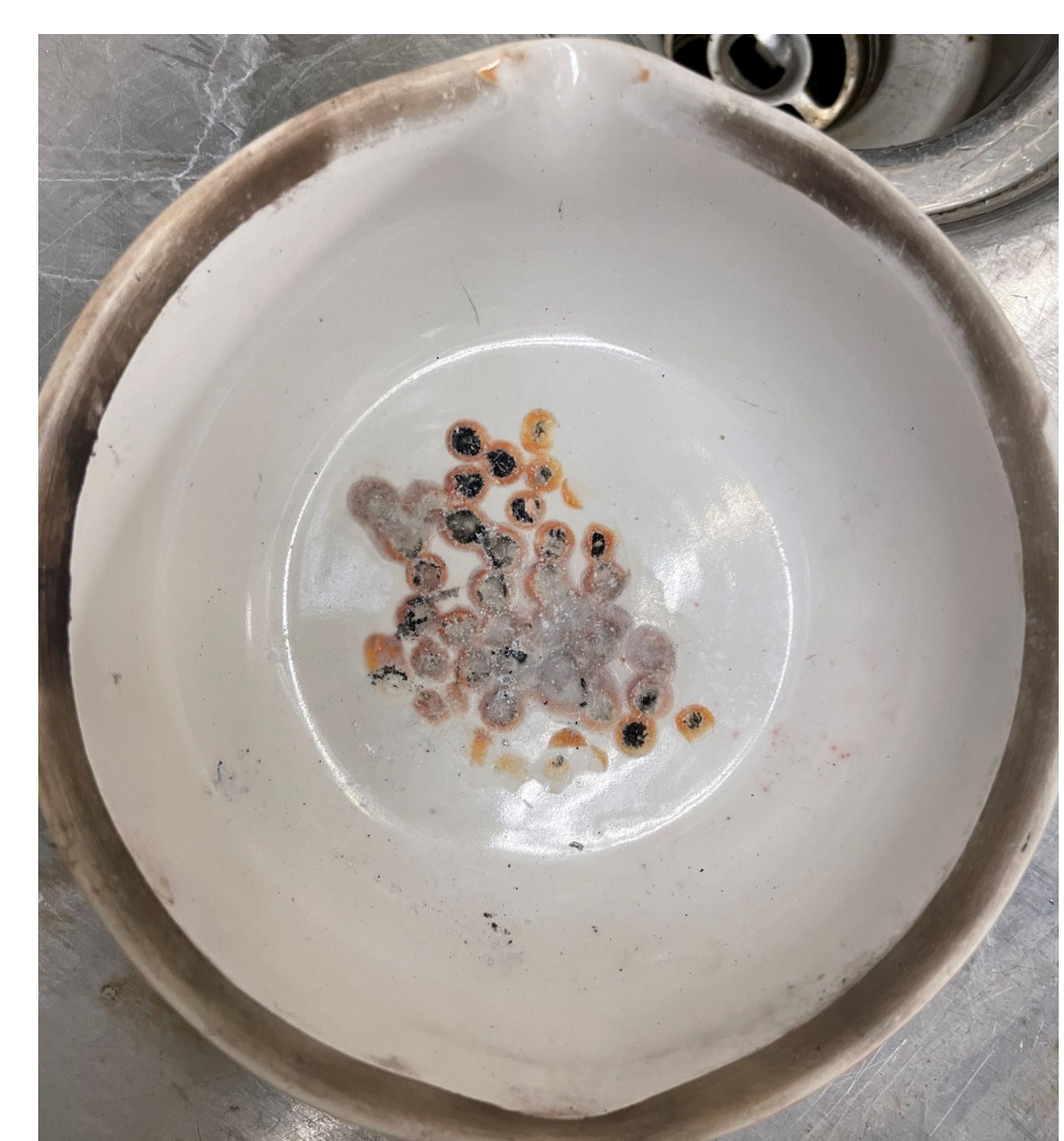
Figure 11. Chemical etching in a ceramic crucible as a result of burning Teflon
