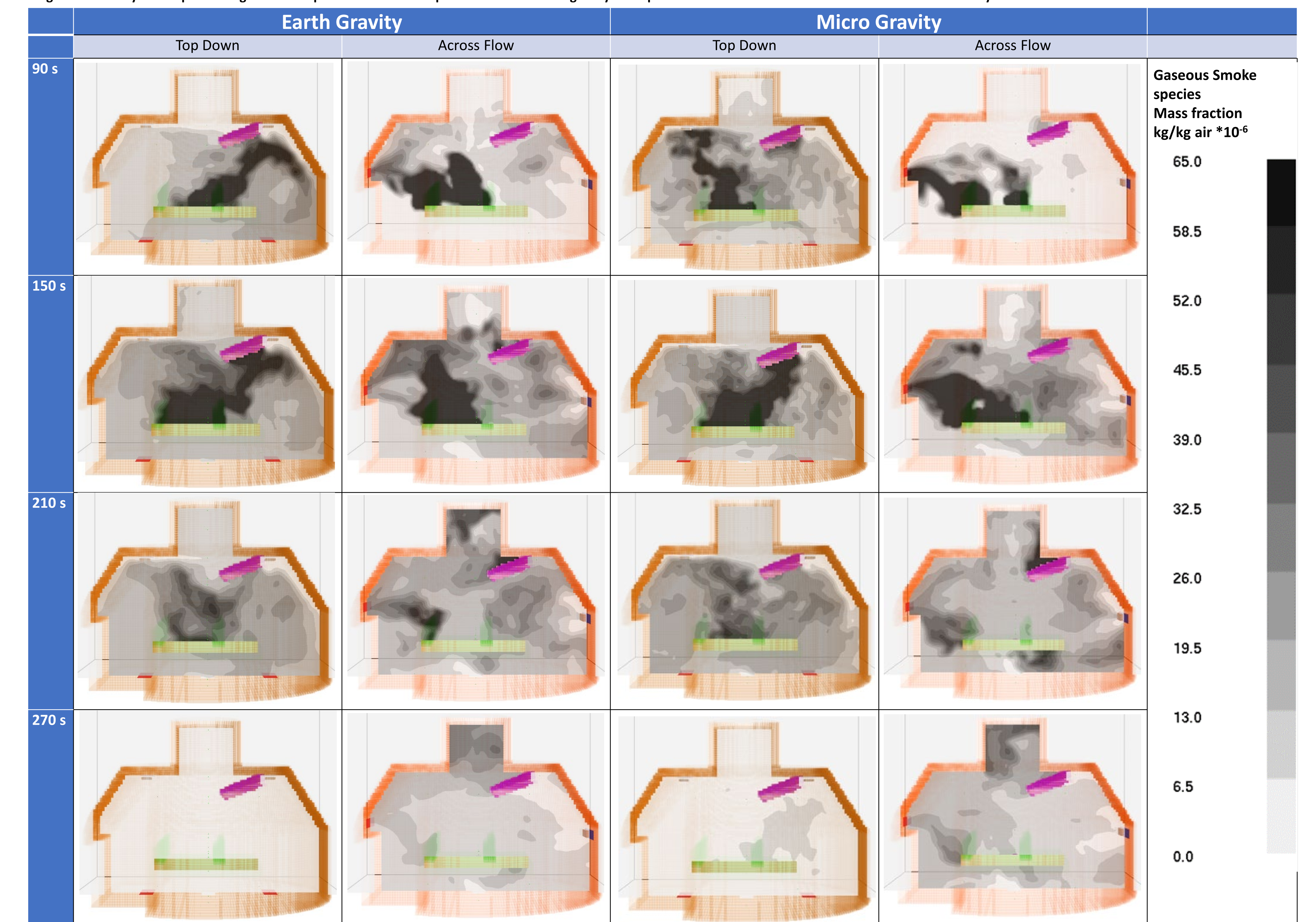
Figure 5: Time evolution of smoke transport for both top down and across flow orientations in Earth gravity and micro gravity.
