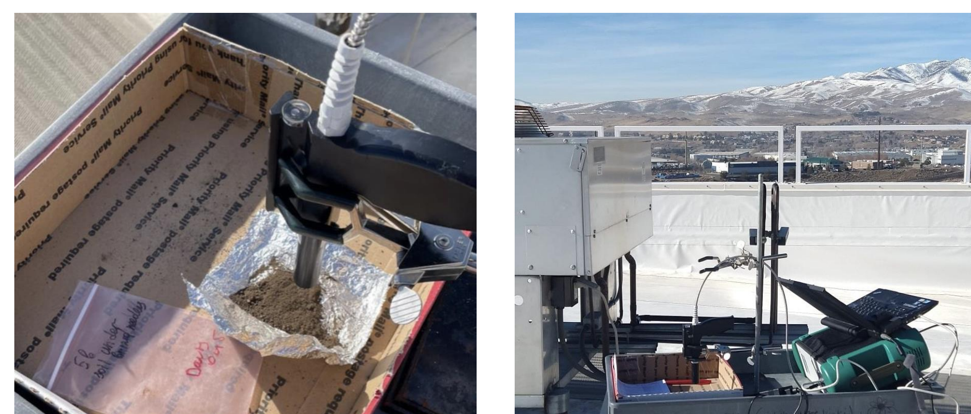
Figure 4. ASD FieldSpec3 set up for acquiring reflectance spectra on DRI rooftop.
