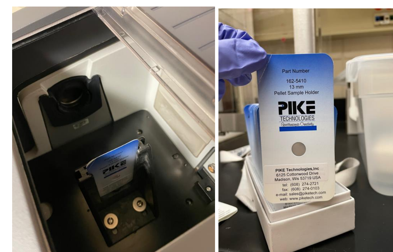
Figure 5. Preparation of pellets of 0.003 g of 0-month, 1-year, and 1.5-year Dixie ash per 0.2 g KBr.
