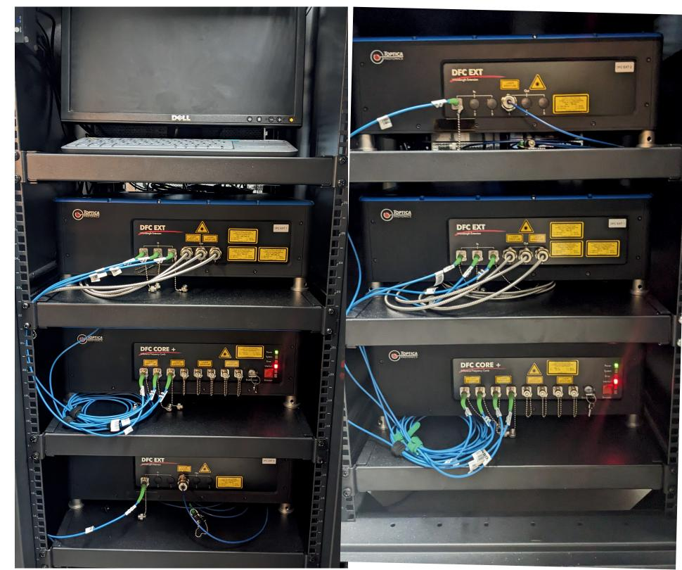
Figure 3- Two DFC+ Cores and wavelength extension modules at UNLV
