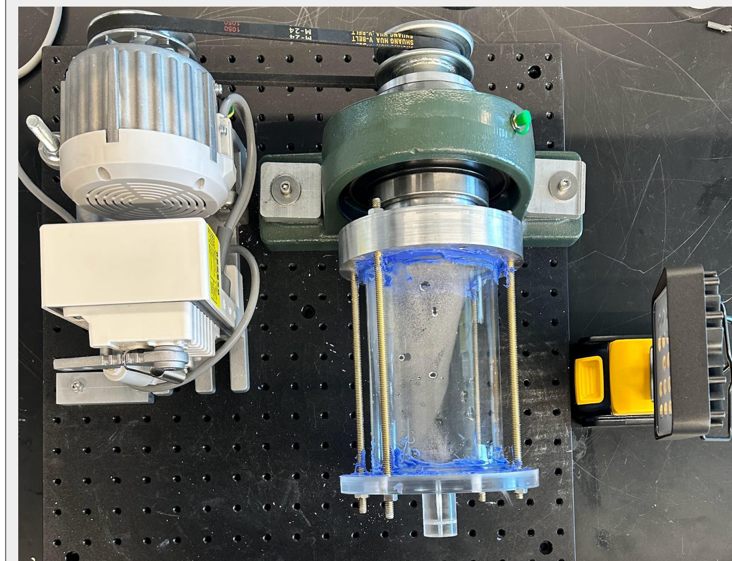
Top view of the experimental setup where the motor on the left turns the acrylic tube containing water. An LED light on the right is used to illuminate the flow within the cylinder.
