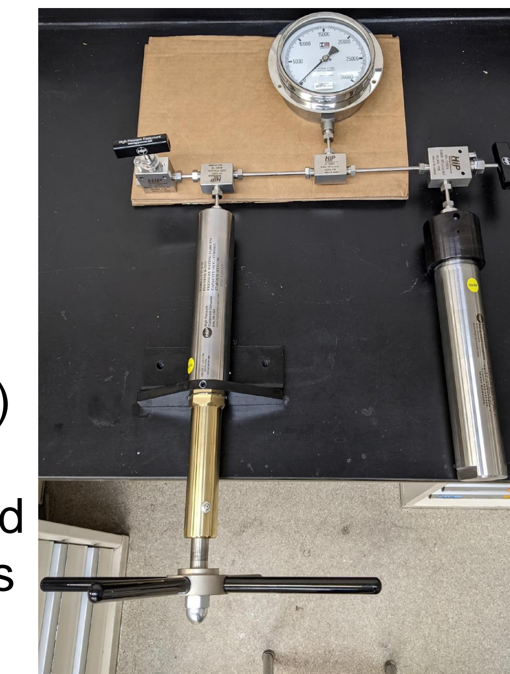
HP vessels pressurized with manual HP pump (0-80 MPa)
