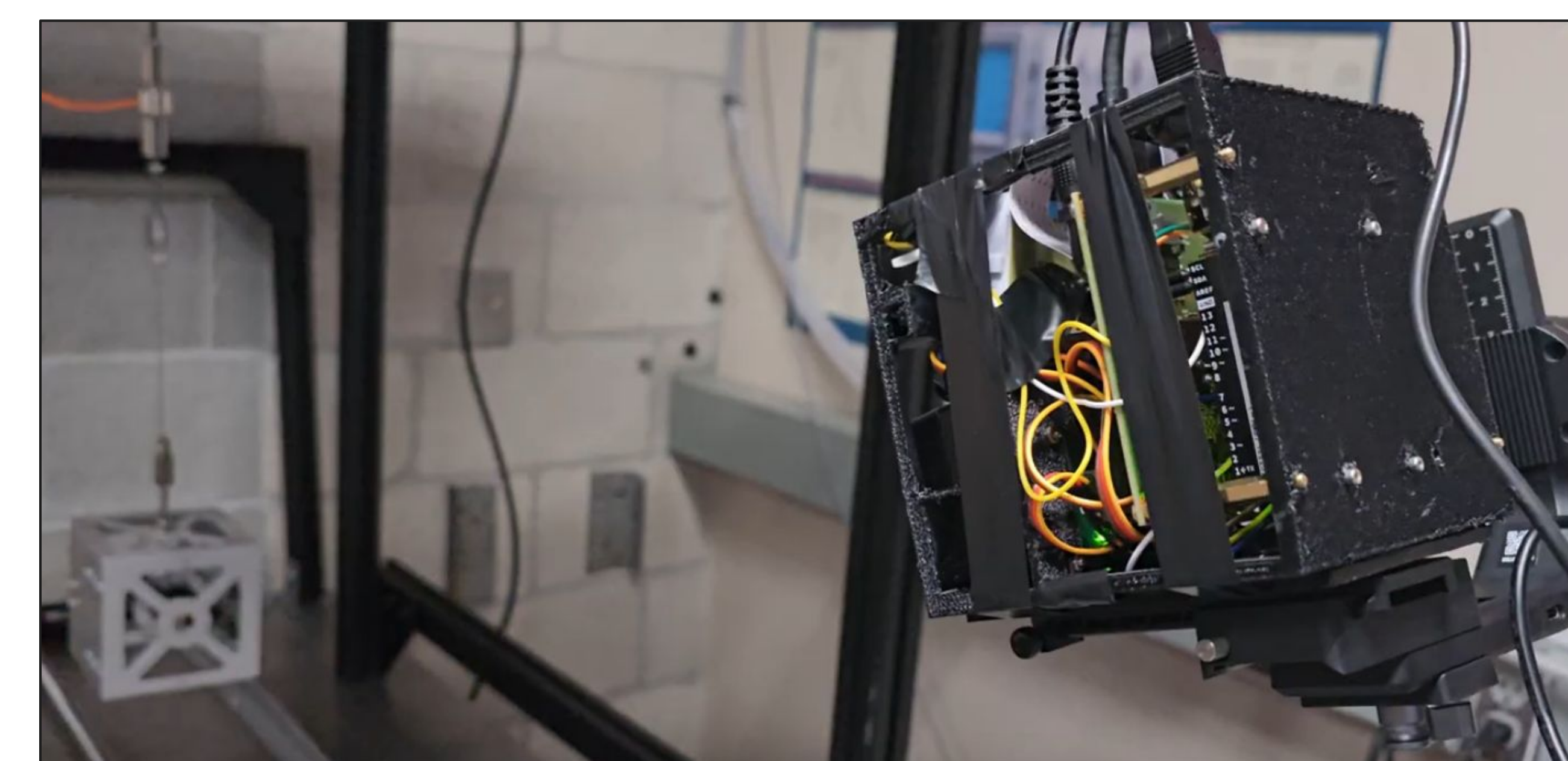
Pictured above is the setup of the CubeSat mounted on the gimbal. Below displays the tracking software (left) and the LIDAR readings (right).
