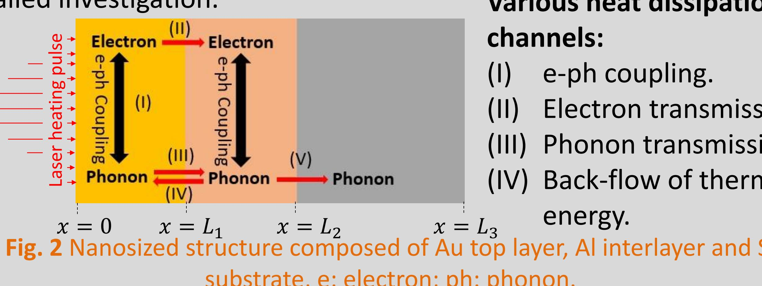
Fig. 2 Nanosized structure composed of Au top layer, Al interlayer and Si substrate, e: electron; ph: phonon.
