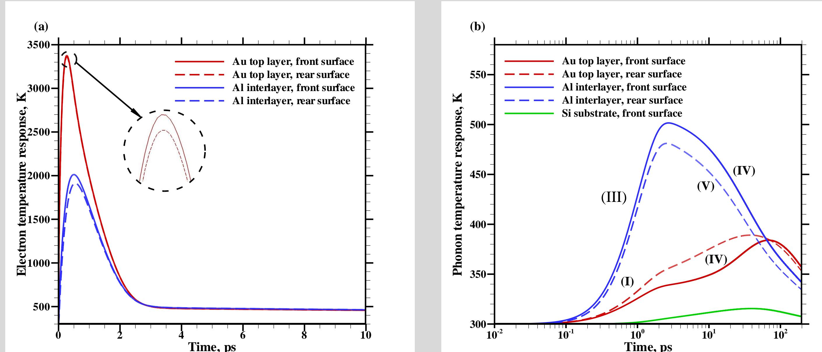
Fig. 3. Electron and phonon temperature response, 10-nm Au/10-nm Al/100-nm Si.
