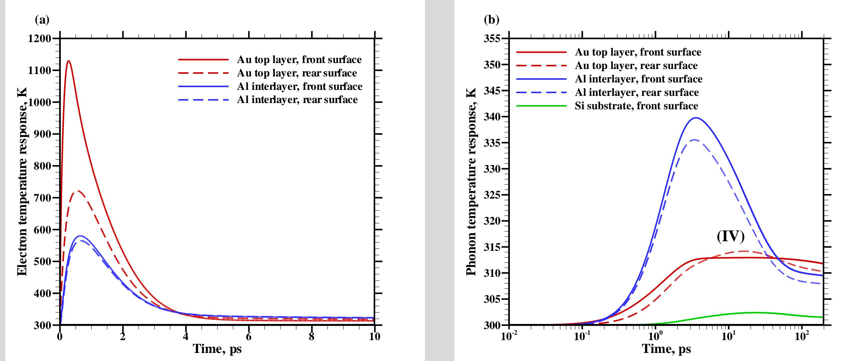
Fig. 4. Electron and phonon temperature response, 200-nm Au/10-nm Al/100-nm Si.
