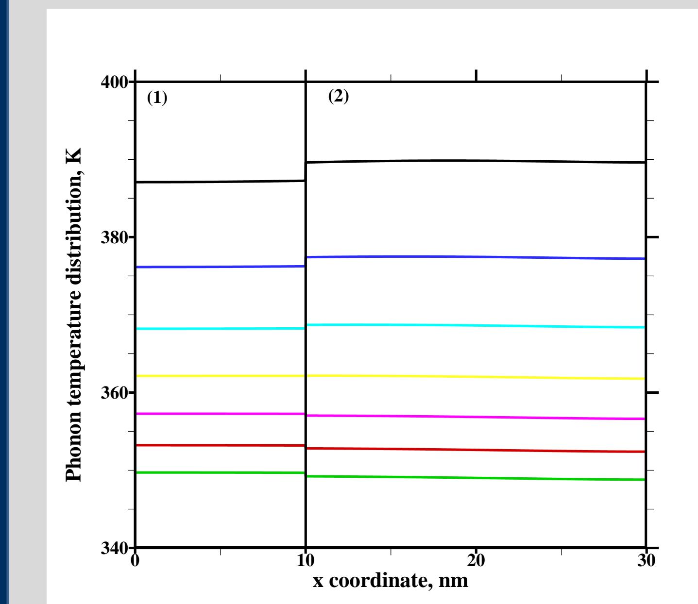
Fig. 6. Electron and phonon temperature distributions, 10-nm Au/20-nm Al/100-nm Si.
