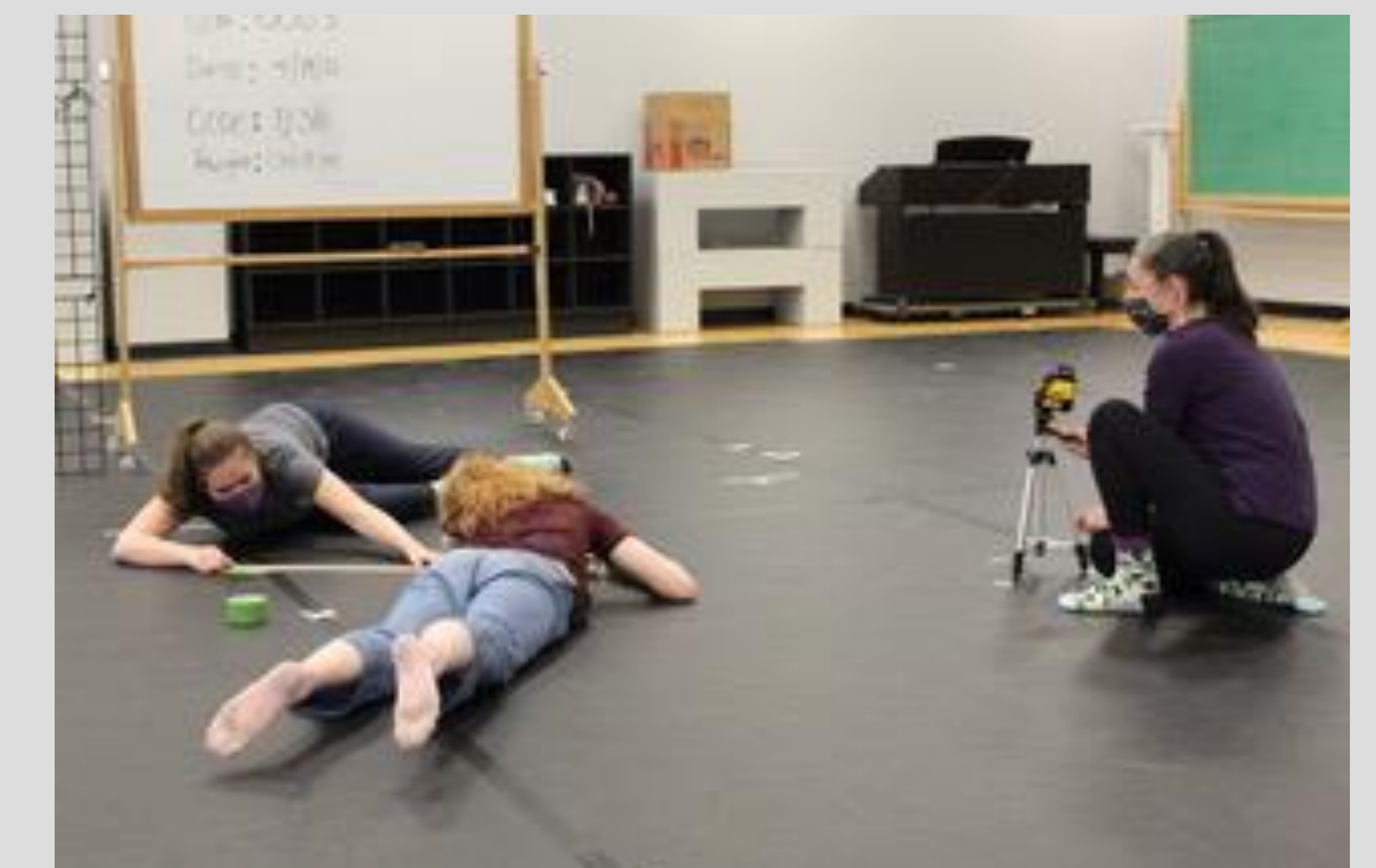
Figure 6: Dayna, Joslyn, and Hannah collecting angle measurements for later comparison to photographic data measurement. The use of a laser level allows us a direct comparison of measurements captured in 3-D space with our 2-D measurements captured using photography. This will ensure accuracy and precision in our data collection and analyses.
